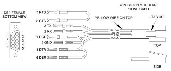
FIGURE 11 - RS-232 CONNECTIONS
